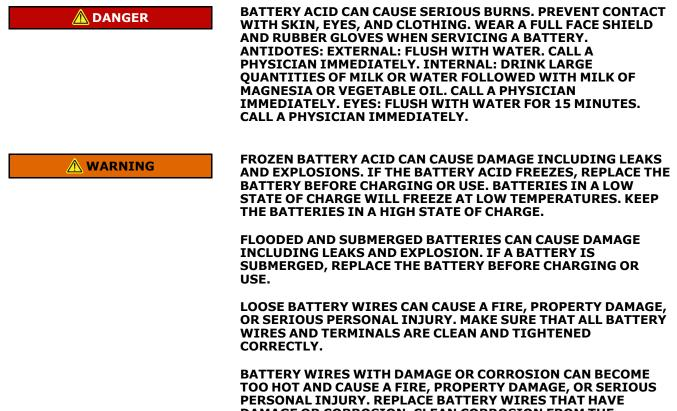
DAMAGE OR CORROSION. CLEAN CORROSION FROM THE BATTERY TERMINALS.
